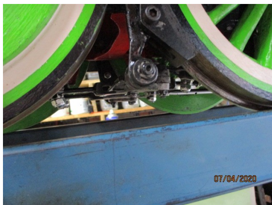
Brake mechanism raised 16mm
